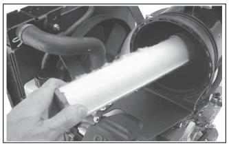
Figure 17. Removing Inner Element.
